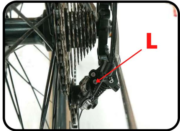
**Step 2** : Now place your chain on the larger sprocket and proceed in the same way to align your roller with your sprocket, this time acting on the lower limit screw (L).
